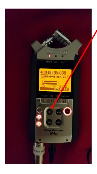
9) At the end of the session, press the stop button on the recorder, and the recording will end. Wait 5 seconds, then power off the unit by sliding the power switch as done in step 3.
