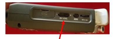
5) Use the REC LEVEL buttons to set the recording level to 45 (this will most likely not need adjusting). The recording level is displayed on the front display panel.
