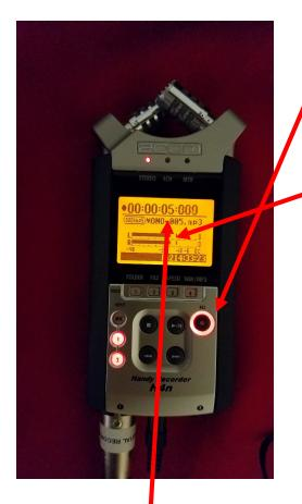
6) Press the REC button once to put the unit into standby mode.
